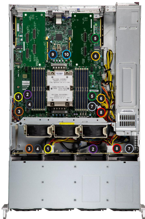
Figure 3-22. Cable Routing Diagram (12 NVMe + 2x PCIe x16)
